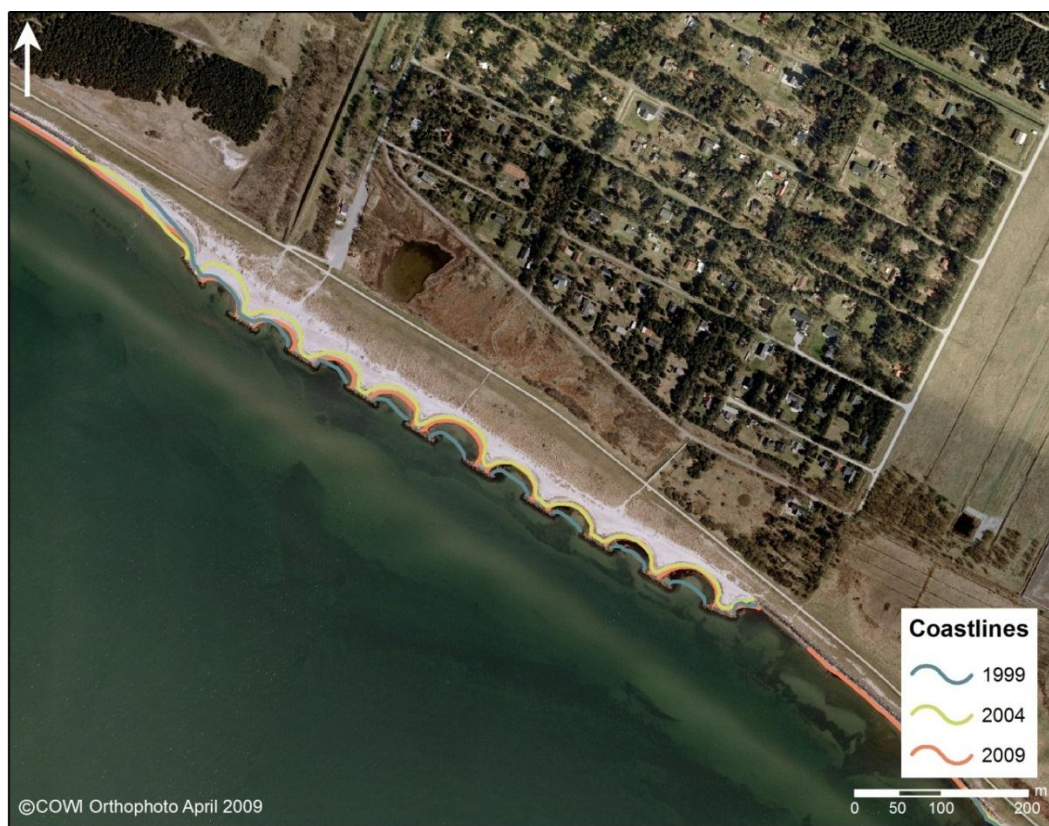
Figure 7.33 Shoreline changes between 1999 and 2009 at Hyldtofte Østersøbad. Aerial photo from 2009 (©COWI Orthophoto April 2009)
