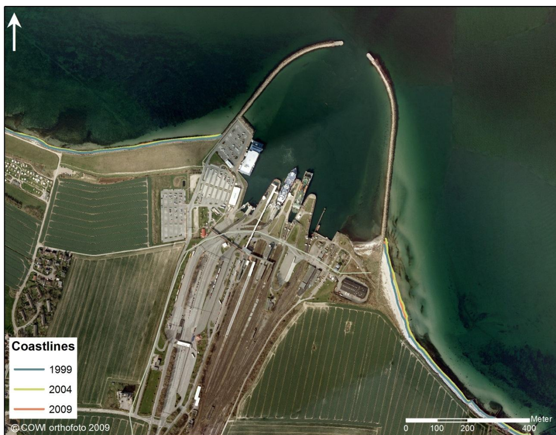
Figure 8.35 Recent shoreline evolution near Puttgarden. Shorelines 1999, 2004 and 2009. Based on analysis of aerial photos, see Section 4.3. Aerial photo from 2009 (©COWI Orthophoto April 2009)
