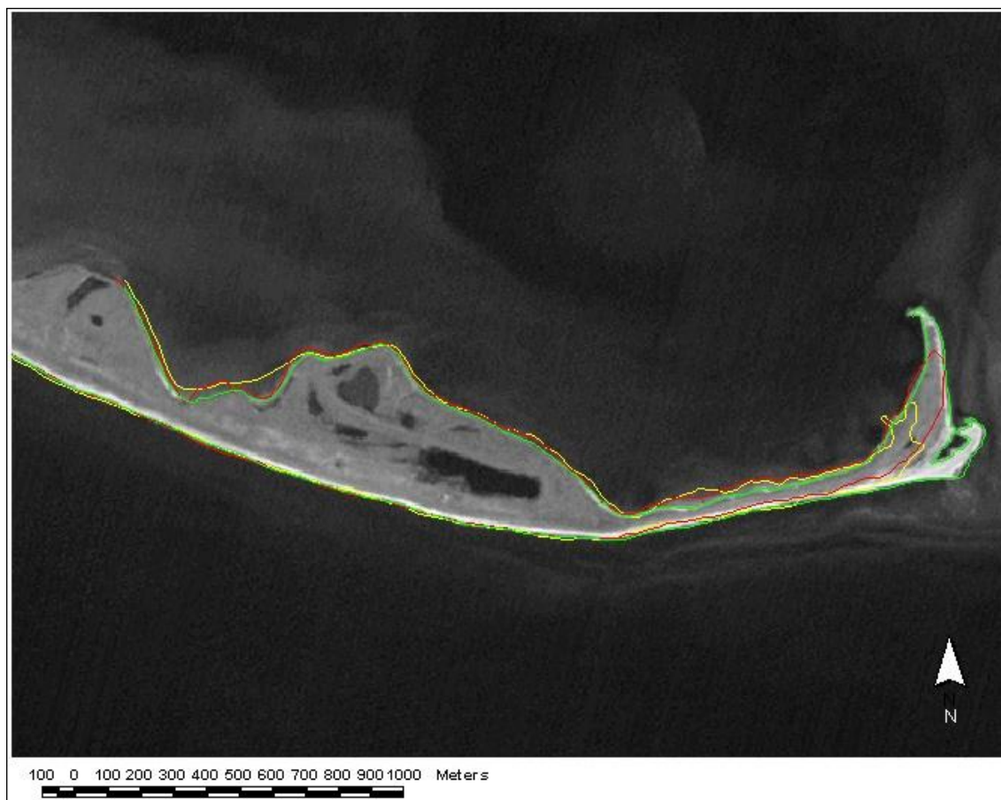
Figure 7.30 Satellite image analysis of the eastern part of Hyllekrog 1973-2003. Background picture dating 2003, marked shorelines: Yellow = 1973. Red = 1986. Green = 2003, from (DHI Water & Environment 2004)
