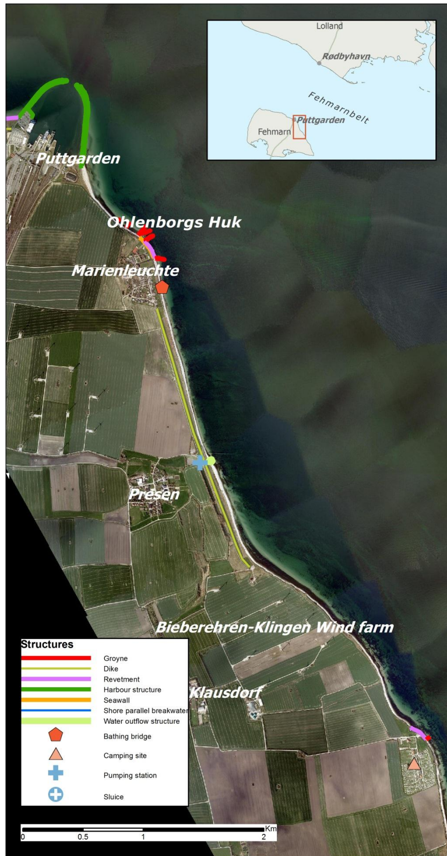
Figure 8.3 Overview of coastline and coastal structures from Puttgarden and Klausdorf. Aerial photo from 2009 (©COWI Orthophoto April 2009). Note: Bieberehren-Klingen wind farm is not the correct name of the wind farm south of Presen.
