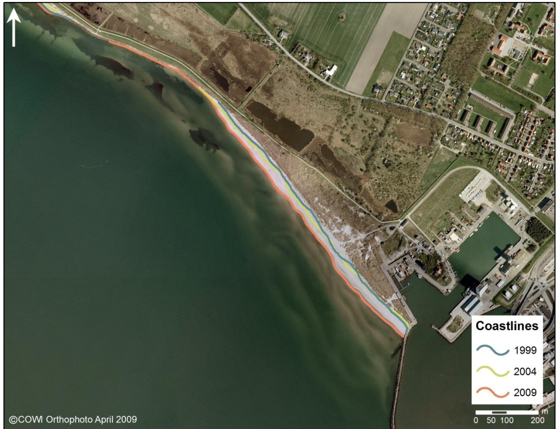
Figure 7.32 Shoreline changes between 1999 and 2009 west of Rødbyhavn. Aerial photo from 2009, (©COWI Orthophoto April 2009)
