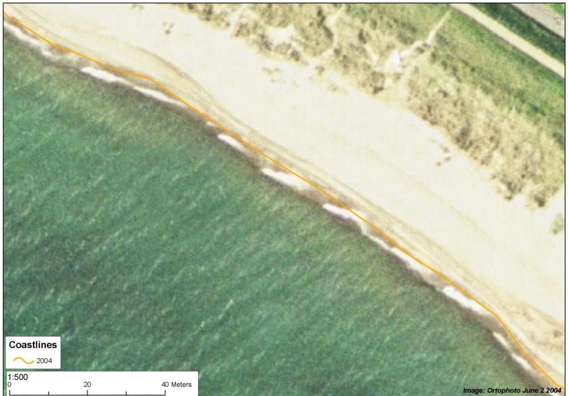
Figure 4.5 Example of digitizing of instantaneous waterline on 2004 image. Aerial photo from 2004 (©COWI Orthophoto Spring/Summer 2004)
