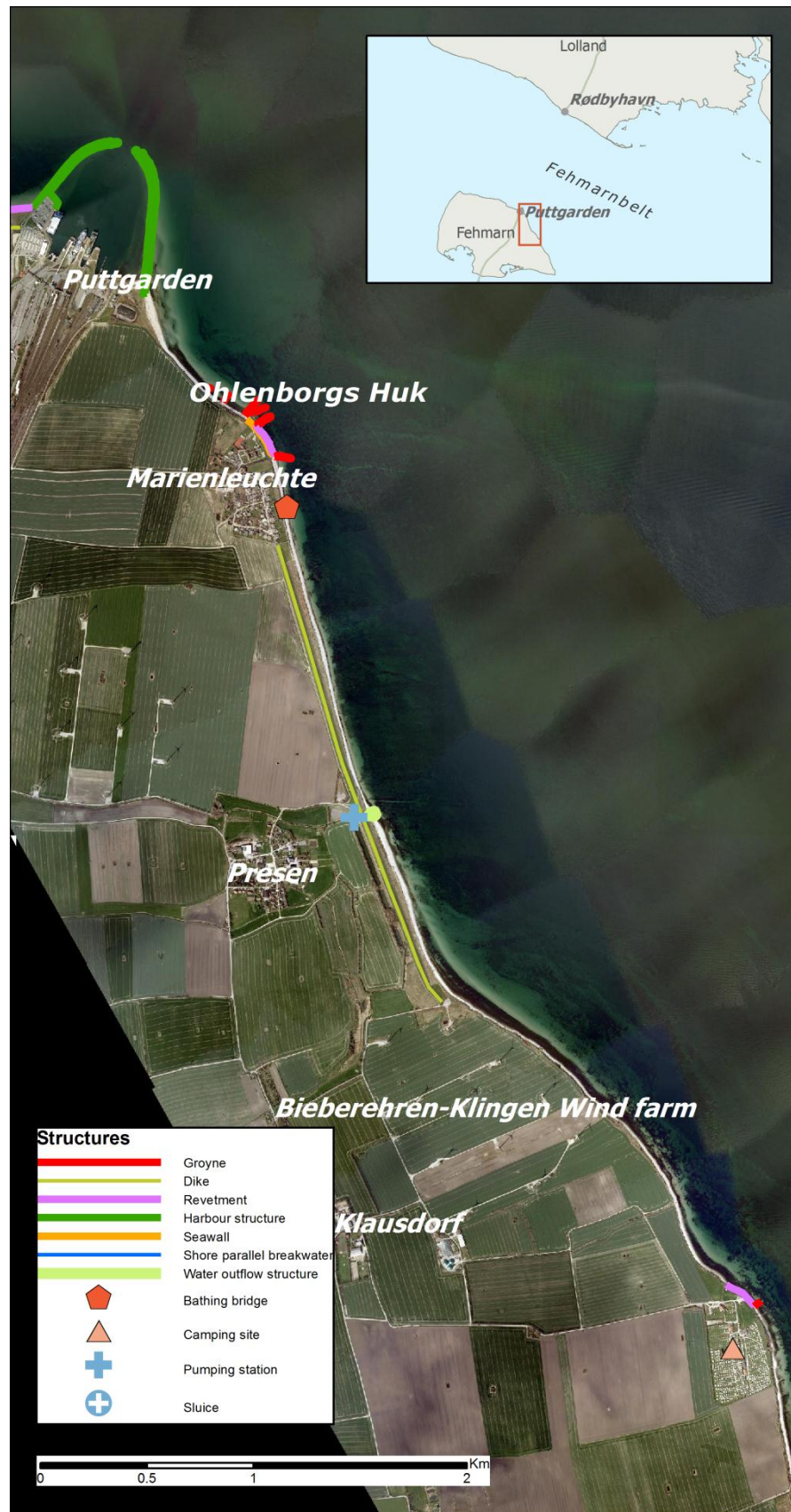
Figure 1.15 Overview of coastline and coastal structures from Puttgarden and Klausdorf. Aerial photo from 2009 (©COWI Orthophoto April 2009). Note: Bieberehren-Klingen wind farm is not the correct name of the wind farm south of Presen
