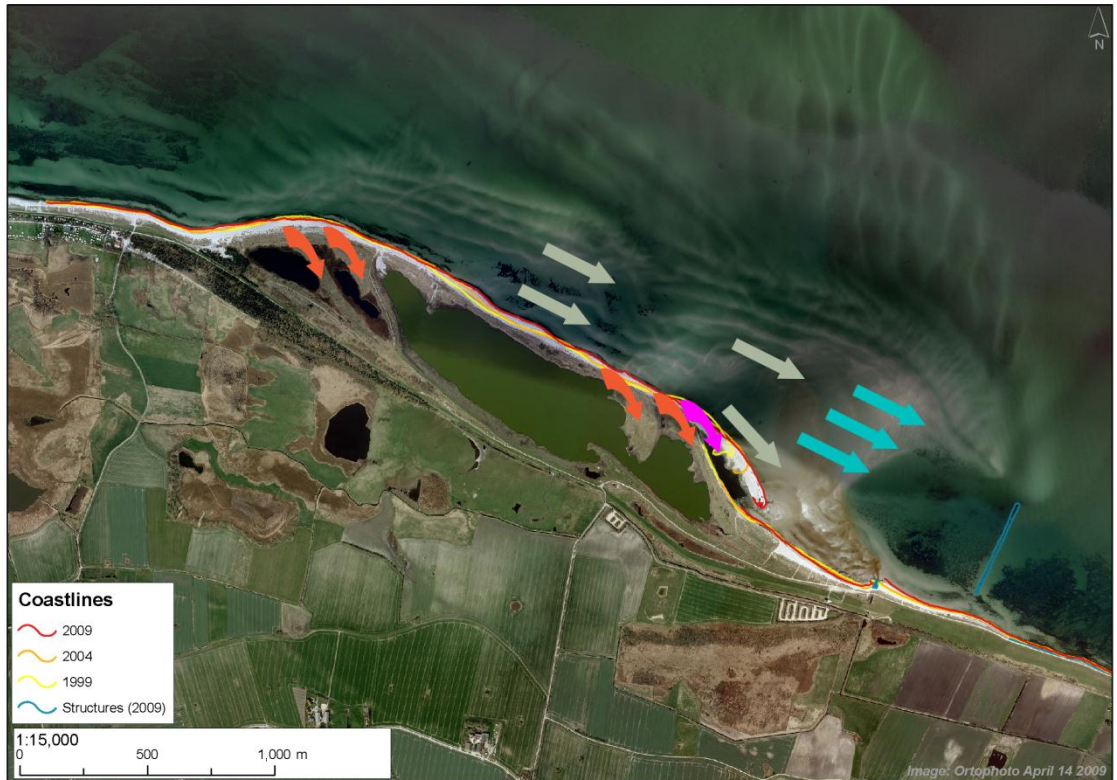
Figure 8.8 Grüner Brink formation with coastlines from 1999, 2004 and 2009., see Section 4.3. Overall morphological development of Grüner Brink indicated with arrows: red arrows indicate remains of old spits. Green arrow indicates present day movement of the spit. Blue arrows indicate progression of the formation below the water level. Grey arrows indicate transport of sediment which deposits on the steep slope or offshore front. Aerial photo from 2009 (©COWI Orthophoto April 2009)
