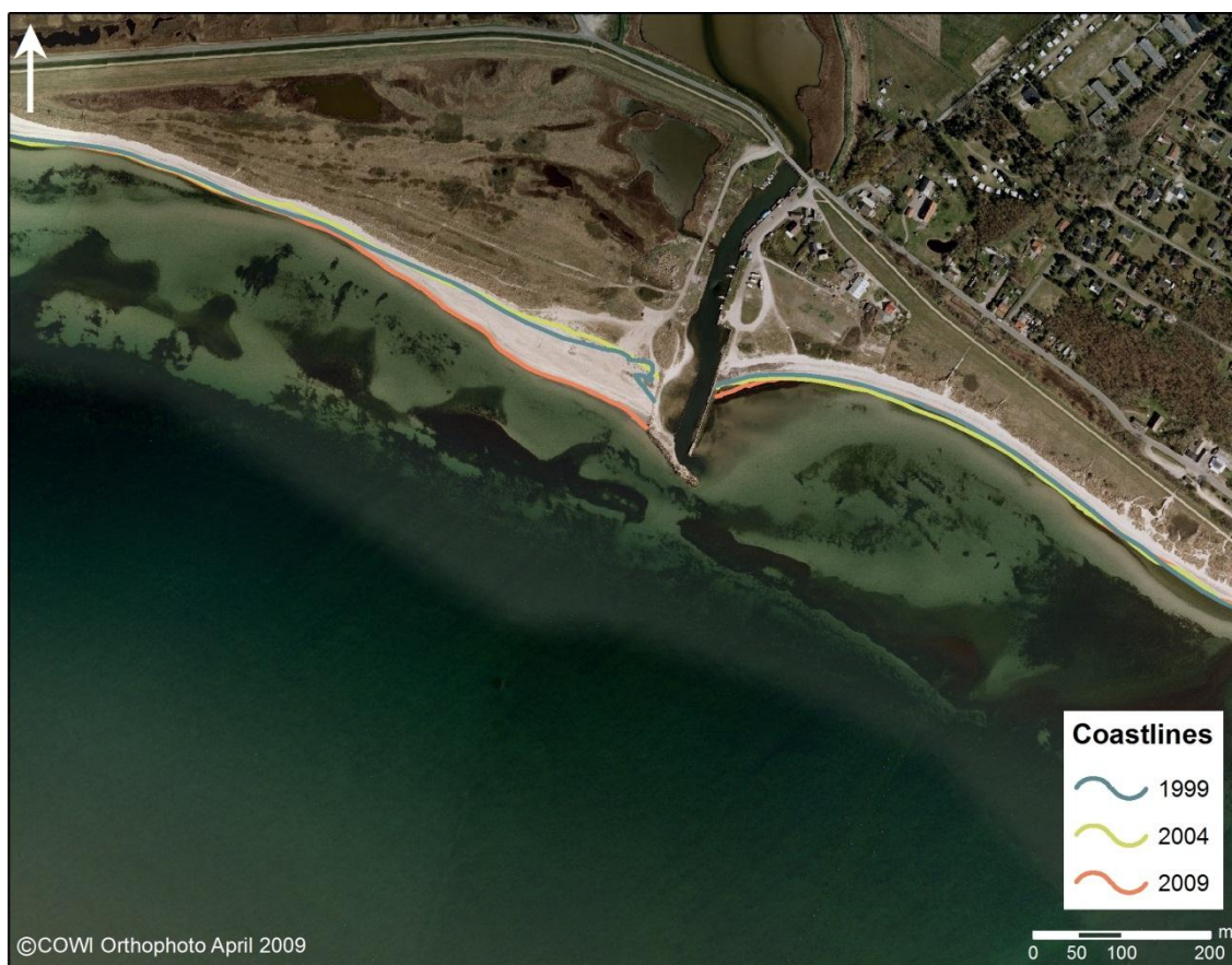
Figure 7.31 Shoreline changes between 1999 and 2009 at Kramnitze. Aerial photo from 2009, (©COWI Orthophoto April 2009)
