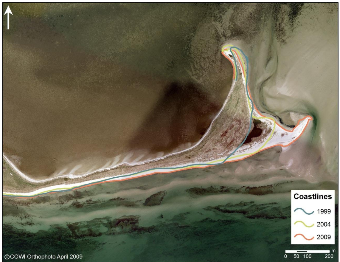
Figure 7.34 Shoreline changes between 1999 and 2009 at Hyllekrog. Aerial photo from 2009 (©COWI Orthophoto April 2009)
