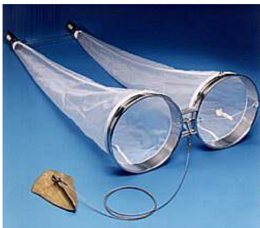
Figure 3.5: A BONGO-net was used to collect fish egg and larvae. Source: www.kc-denmark.dk
