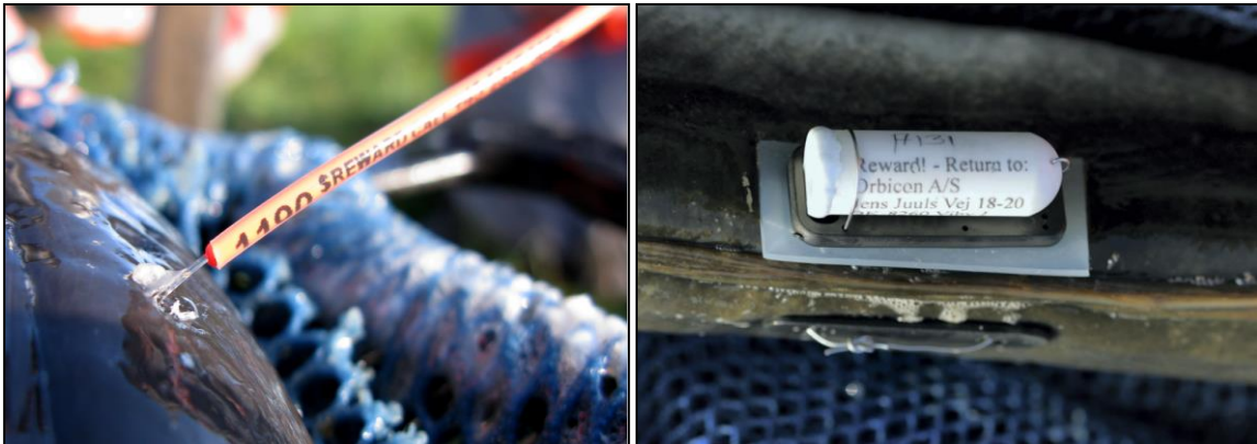
Figure 3.15: Left: A Hallprint T-bar tag with contact information text. Right: The DST (Data Storage Tag) with return information text. The sensors of the DST store information on temperature and depth at user-defined time intervals. © Christian B. Hvidt.
