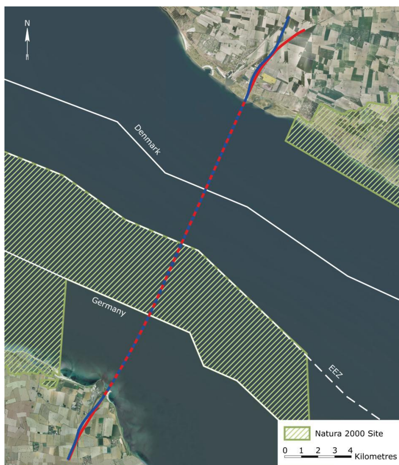
Fig. 2.1 Conceptual design alignment for immersed tunnel E-ME (August 2011)
